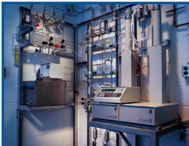
This chemical reactor system was created by Pacific Northwest National Laboratory for developing and optimizing processes to make value-added chemical products from basic chemicals derived from renewable feedstocks.
