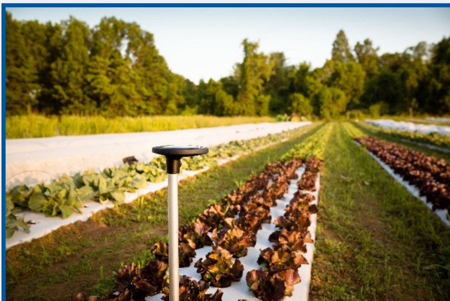
The Arable Mark monitors crop growth and weather to inform farm management and breeding. Photo Credit: Arable Labs Inc.
