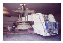
Nine-meter centrifuge at the Center for Geotechnical Modeling at UC Davis, a host facility in the Network for Earthquake Engineering Simulation, funded by the National Science Foundation.
