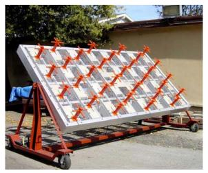
A single panel of 32 dipole antennas for the Advanced Modular Incoherent Scatter Radar (AMISR). AMISR consists of three antenna faces, each containing 128 of these panels. *Credit: SRI International*
