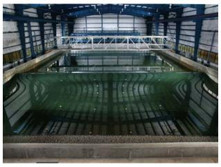
The NEES Tsunami Wave Basin is pictured above. Located at Oregon State University, it is the world's largest shareduse research facility for the study of effects of tsunami inundation on coastal buildings and lifeline infrastructures. A solition (or solitary wave) is being demonstrated in this photo. *Credit: Kelly James, Oregon State*
