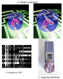
Electronic nose detecting a chemical and a photograph showing the actual size of the device. Credit: Nathan Lewis, California Institute of Technology
