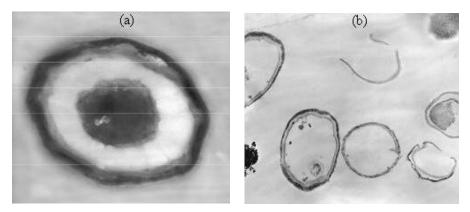
Transmission electron microscopy image of bacillus spores before (left) and after (right) photocatalytic treatment by visible light-illuminated metal doped TiON. *Credit: Mark Shannon, University of Illinois.*
