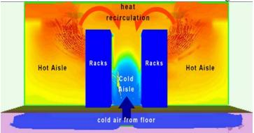
Figure shows the heat recirculation effect in a typical data center using a cold aisle – hot aisle configuration. *Credit: Image generated in the Arizona State University Impact lab using the Flovent Computation Fluid Dynamics (CFD) software.*
