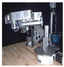
Mockup of integrated inspection and robotic turbine blade finishing system. *Credit: Western Robotics.*
