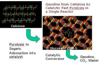
In one reactor, cellulose is broken up into sugar fragments that interact with a catalyst to become aromatic compounds used for gasoline. *Credit: George Huber, University of Massachusetts at Amherst.*
