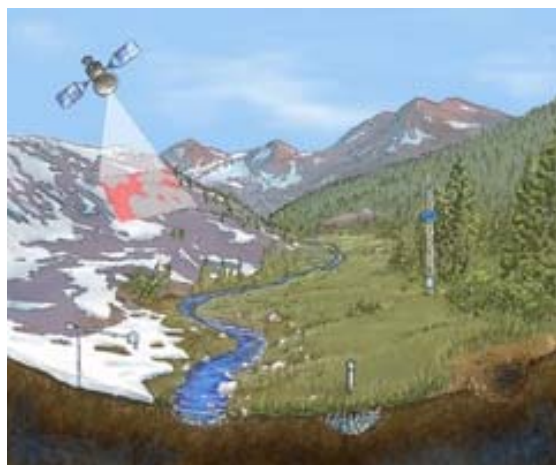
Schematic vision of a Critical Zone Observatory, showing part of the multiple sensor array that will be used to investigate the hydrological, geochemical, geobiological, and physical evolution of the critical zone. Methods brought to bear by multiple investigators and institutions will range from detailed field surveys to computationally intensive numerical modeling, from geophysical and geochemical investigations to networked cyberinfrastructure that will share and archive an unparalleled data type. Credit: Roger Bales, UC Merced.
