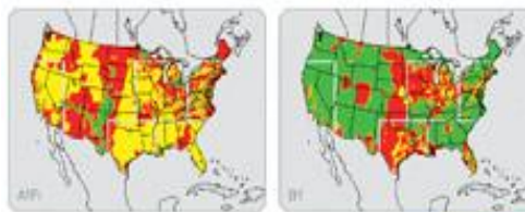
Relative contributions (percent) of the projected emissions (EMS) and climate (MET) changes to total surface ozone concentration trends between 2050 and 1998: A1Fi scenario and B1 scenario. Green denotes the dominance of the EMS effect (contribution greater than 70 percent), yellow denotes the MET effect (contribution greater than 70 percent), and red denotes where both effects are deemed to be important. Credit: Xin-Zhong Liang, University of Illinois at Urbana-Champaign.
