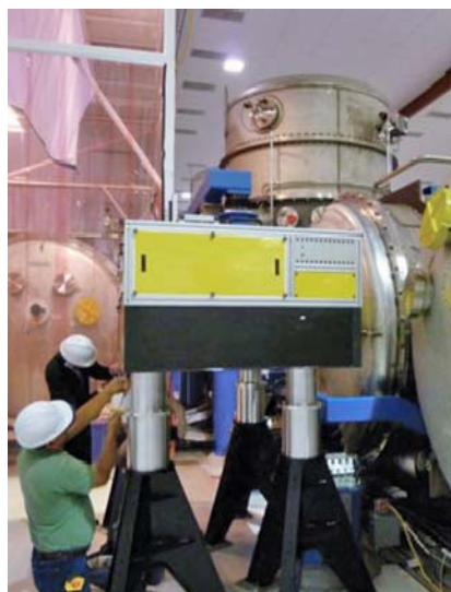
Installation of a quantum-mechanical squeezing experiment at LIGO in 2011. The temporary experiment allowed LIGO to increase its sensitivity by more than 20% over most of its frequency range. Such research is conducted by LIGO Laboratory and the LIGO Scientific Collaboration to reduce risk in the Advanced LIGO construction project. Credit: Caltech/MIT LIGO Laboratory.
