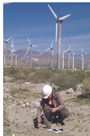
A student volunteer prepares to deploy a sensor on a wind farm near Palm Springs, California, that will record high-frequency seismic waves for the Salton Sea Imaging Project. Principal Investigators: John Hole, Virginia Tech, Joann Stock, Caltech, and Gary Fuis, USGS. Credit: IRIS.
