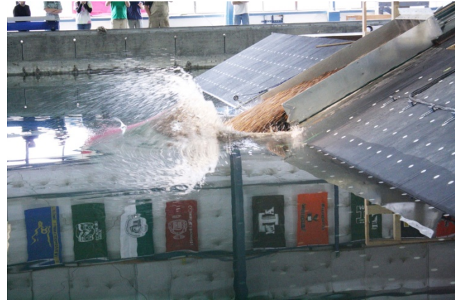
Using a unique landslide tsunami generator, researchers at the Georgia Institute of Technology in cooperation with faculty at University of Alaska at Fairbanks are investigating a methodology for improved assessment and mitigation of landslide and tsunami hazards. Field data from landslide-generated tsunamis events are limited to very few cases with marginal data that are generally missing the most important information related to tsunami generation characteristics. Researchers are compensating for this lack of field data by creating physical models of three-dimensional tsunami generation by deformable landslides and source run-up in the NEES Tsunami Wave Basin at Oregon State University. Credit: Devin K. Daniel, California Polytechnic State University, San Luis Obispo, NEES summer 2010 REU student
