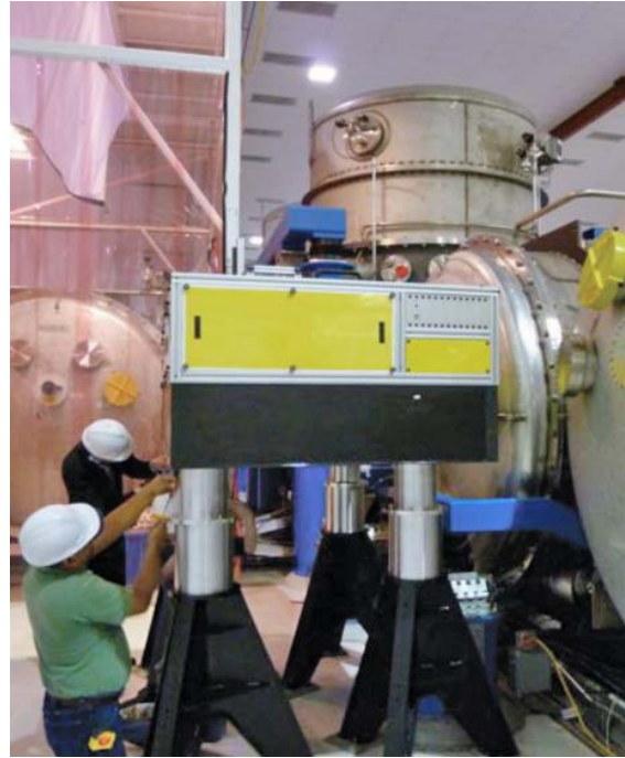
Installation of a quantum-mechanical squeezing experiment at LIGO in 2011. The temporary experiment allowed LIGO to increase its sensitivity by more than 20 percent over most of its frequency range. Such research is conducted by LIGO Laboratory and the LIGO Scientific Collaboration to reduce risk in the Advanced LIGO construction project. Credit: Caltech/MIT LIGO Laboratory.
