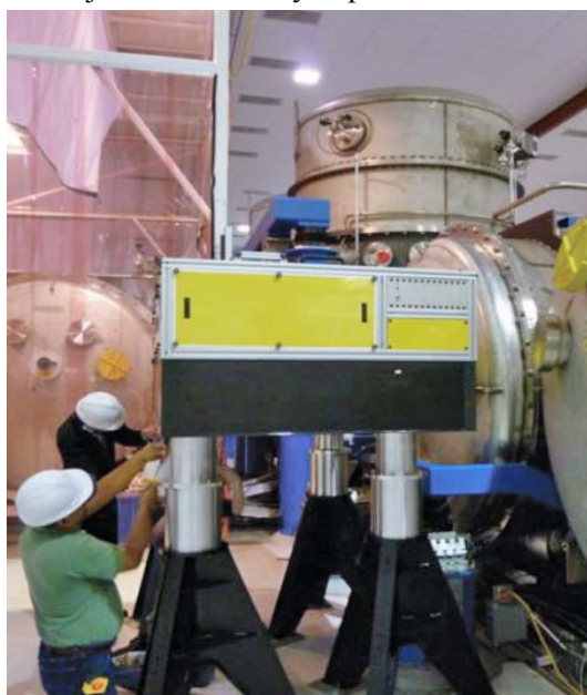
Installation of a quantum-mechanical squeezing experiment at LIGO in 2011. The temporary experiment allowed LIGO to increase its sensitivity by more than 20 percent over most of its frequency range. Such research is conducted by LIGO Laboratory and the LIGO Scientific Collaboration to reduce risk in the Advanced LIGO construction project. Credit: Caltech/MIT LIGO Laboratory.
