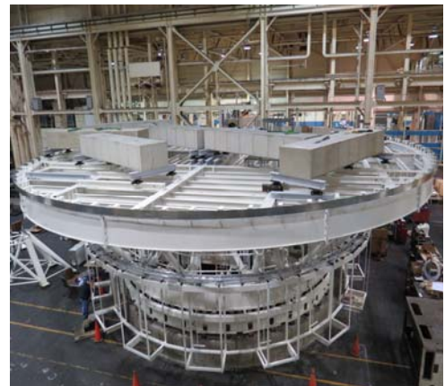
The Coudé Rotator loaded down with dummy masses for final acceptance testing. Credit: M. Warner, DKIST.
