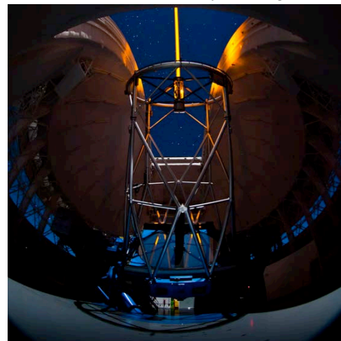
The laser at Gemini-South produces synthetic guide stars on the sky, which the GeMS adaptive optics system uses to correct wide-field images for atmospheric turbulence. Credit: Gemini/AURA.
