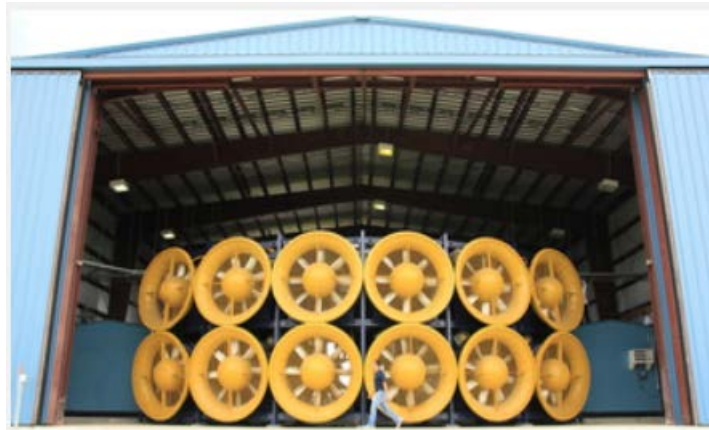
The 12-fan Wall of Wind at Florida International University (FIU), one of the NHERI experimental facilities, will enable better engineering against tornadoes, hurricanes, and other windstorms. Photo Credit: Courtesy of FIU.
