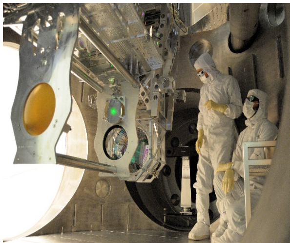
Installation of the green (532nm) Arm Length Stabilization (ALS) subsystem for AdvLIGO. Credit: Caltech/MIT LIGO Laboratory.
