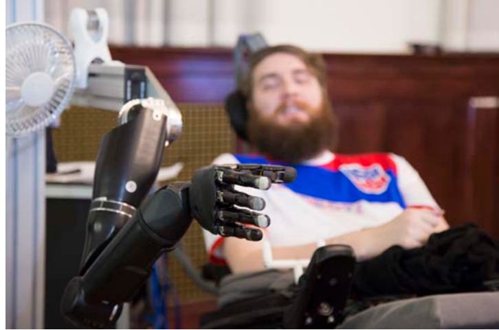
A man manipulates a robotic arm via a computer chip in his brain.
