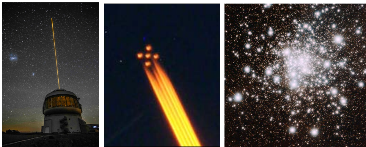
The Gemini South telescope in Chile firing its laser into the night sky (left). The laser produces a “constellation” of five synthetic guide stars (center) that are used to correct for atmospheric blurring. The Gemini observation (on the right) of a Globular Cluster shows an example of an image sharpened in this way. Credit: Gemini Observatory/NSF/AURA.
