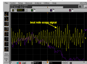
(B) Comb offset error signal generation
