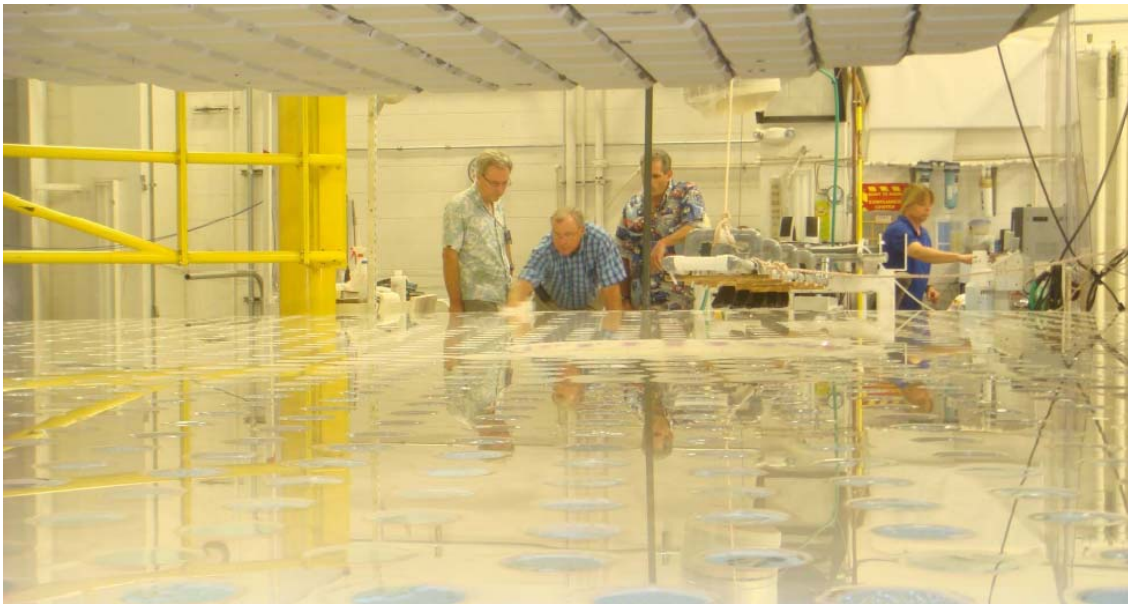
Back surface inspection after final polish
