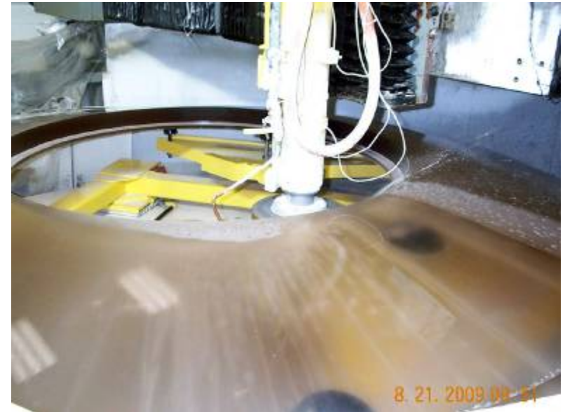
Grinding inside bevel before acid etching
