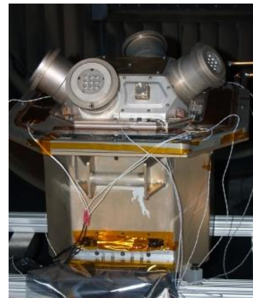
ST-7 flight design microcolloid thruster assembly
