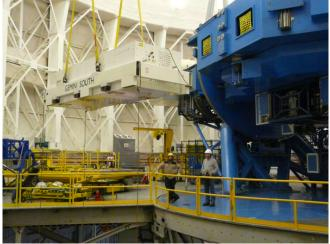
50-watt laser (above) is projected as a 5-spot constellation covering 1 sq. arcmin by GeMS to illuminate the sodium layer ~90 km above Cerro Pachon, Jan. 22, 2011.
