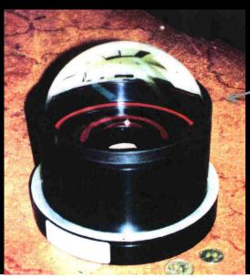
Design, then build, novel wide-field imager, with first-generation 1K x 1K CCD chip.
