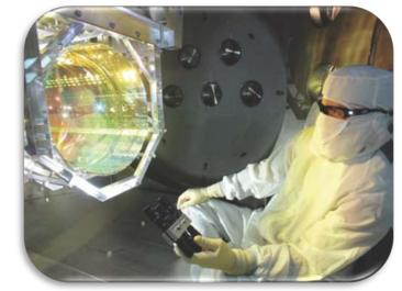
Improved mirror coatings: will reduce Brownian thermal fluctuations in the middle of the frequency range
