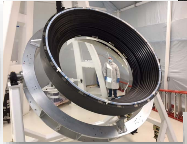
L2 lens coated and assembled in its structure
