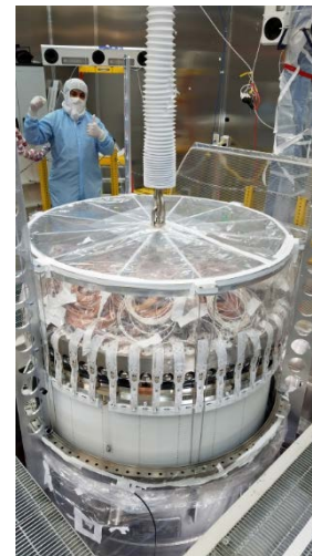
Sept. 2019: TPC assembled, then inserted into inner cryostat vessel.
