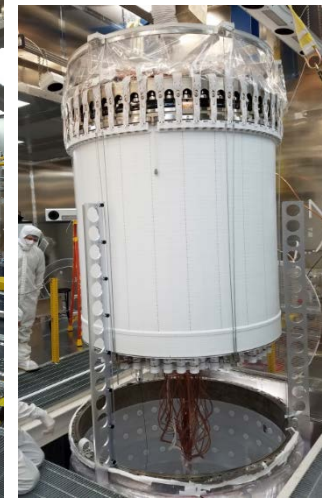
Sept. 2019: TPC assembled, then inserted into inner cryostat vessel.
