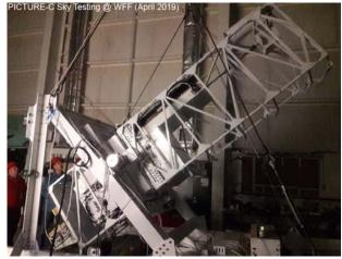
PICTURE-C - Chakrabarti/Univ. of Mass.) will image five nearby star systems to search for dust and debris disks. PICTURE-C will demonstrate a balloon-based clear aperture telescope with low order wave front control, high performance vector vortex coronagraph, and a microwave kinetic inductance detector.
