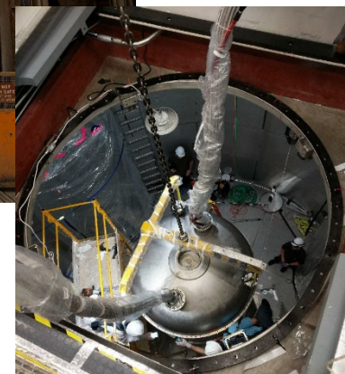
TPC/ICV inside OCV in water tank (Dec. 2019)
