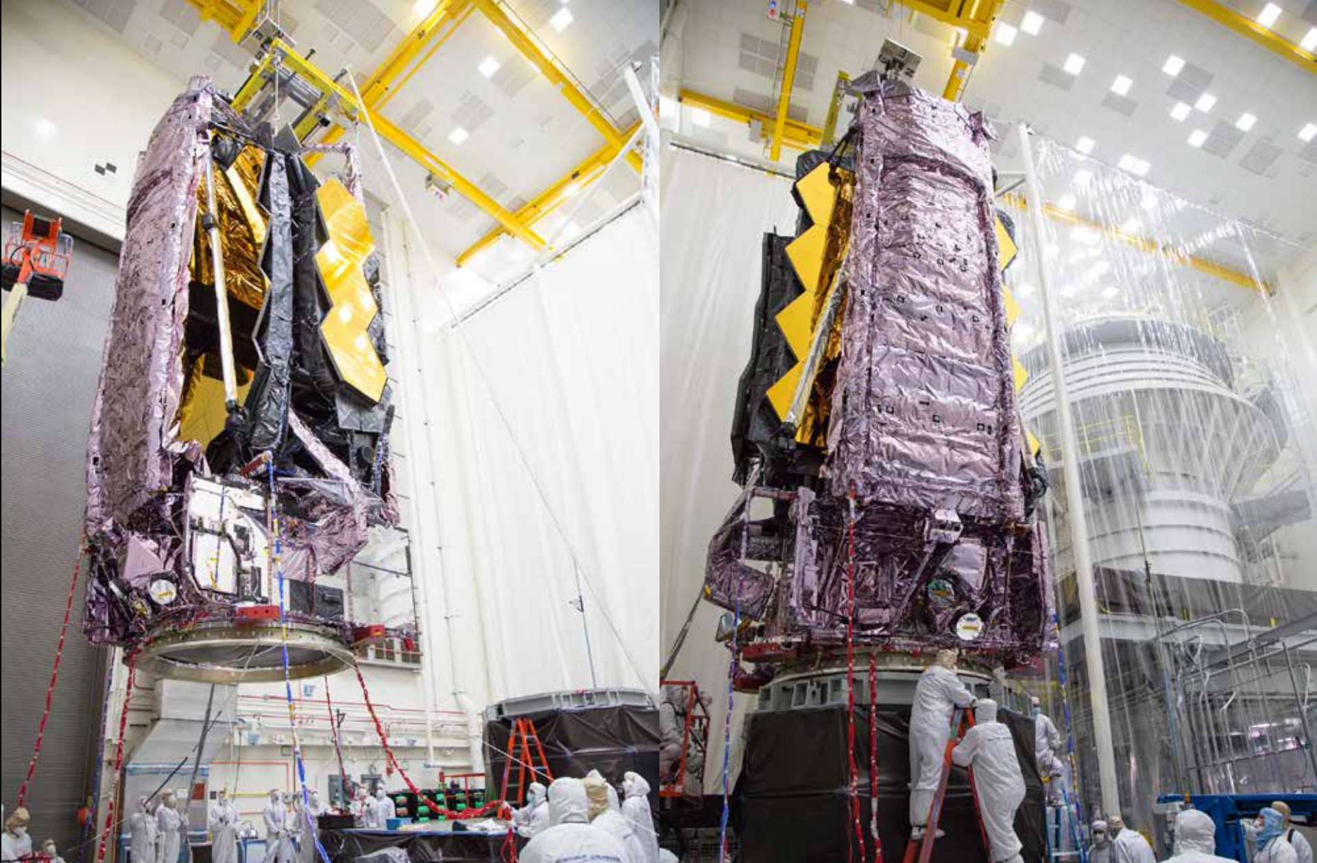
The fully assembled and folded James Webb Space Telescope on the vibration table at Northrop Grumman Space Park (September 2020). This is the configuration that Webb will be in when it is mated to the Ariane 5 launch vehicle in 2021.
