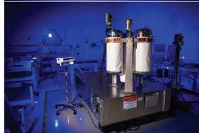
Mirror Module Assembly (MMAs) Integrated on MMSS Deck
