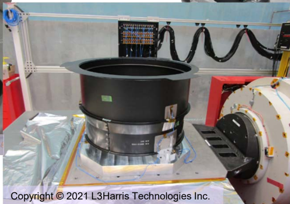
OTA Secondary Mirror baffle & shade sine vibration test
