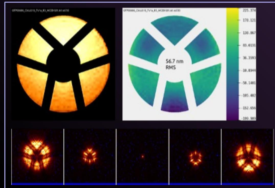
*Phase retrieval shows wavefront error at cold temperature significantly better than required*
