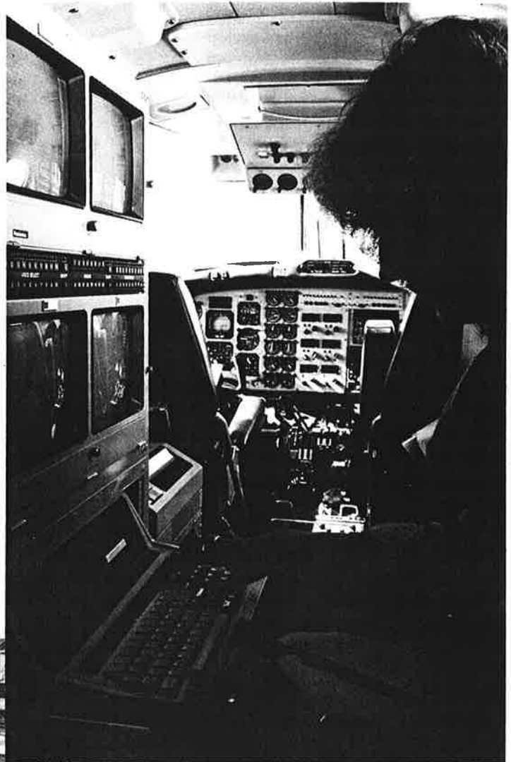
King Air interior. NCAR's King Air is a versatile research aircraft that can be readily adapted for individual flight missions to study the atmospheric boundary layer, air-sea interactions, air chemistry, and cloud physics. Put into service in April 1983, it is equipped with a compact data system that incorporates a dual computer system with an interactive terminal and four on-board video displays.
