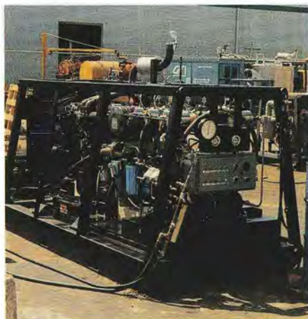
Life-saving equipment. An ultrahigh-pressure pump and jet lance, similar to what is shown here, powered the waterjet rock-cutting system used to free Jessica McClure from a well in Midland, Texas. NSF was instrumental in early funding of the research that produced the ultrahigh-pressure nozzles and related technology used in the rescue. Second photo shows pump that is inside large box.
