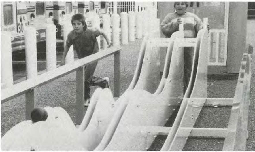
The friction factor. In this exhibit, two balls race down a circular track; one is partially filled with sand and the other is solid. Because of internal friction, the sand-filled ball soon stops accelerating and the solid ball always wins the race.
