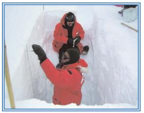
*NSF CReSIS investigators conduct snow pit measurements for radar survey in Antarctica.*
