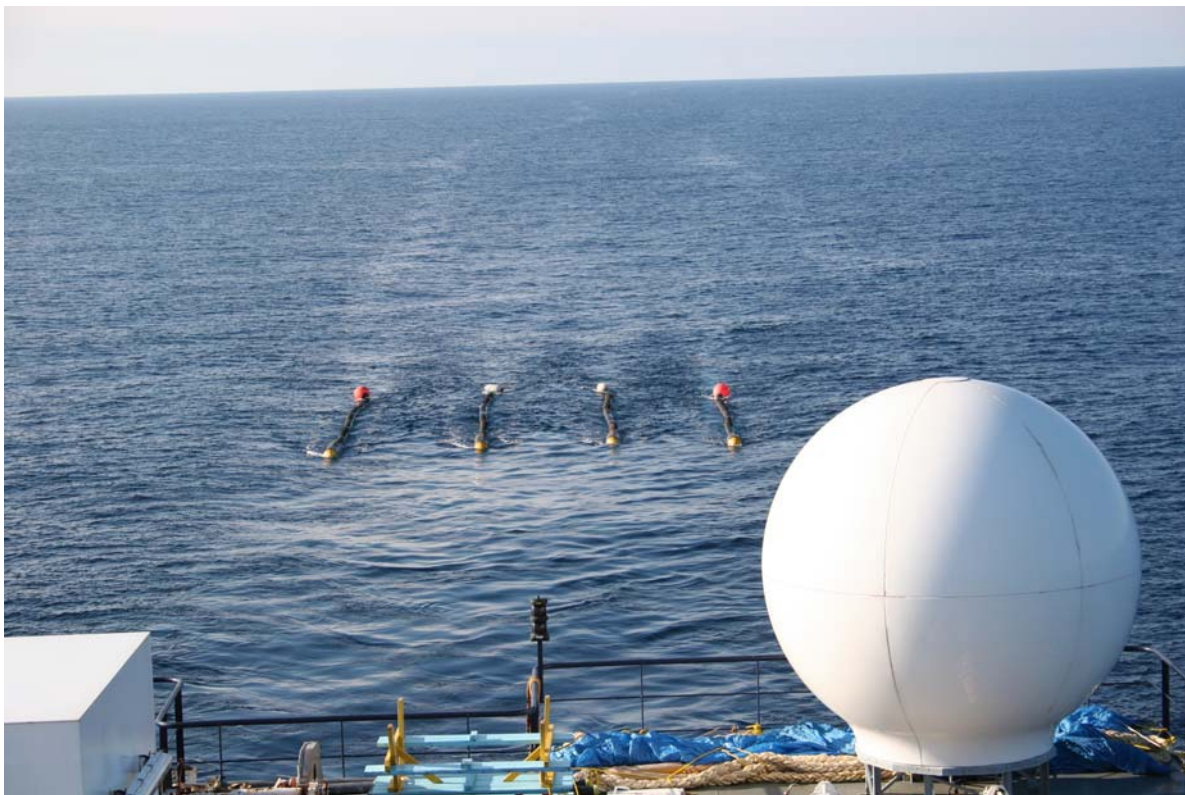
FIGURE C.2. View off the stern of the R/V Marcus G. Langseth when the 4-string airgun array was towed.
