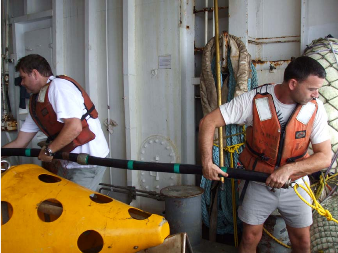
FIGURE D.1. Deployment of the PAM hydrophone streamer from the stern of the R/V Marcus G. Langseth .
