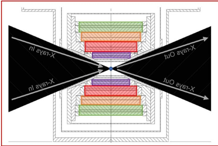
To build a dedicated High Magnetic Field (HMF) X-ray Beamline at the Cornell High Energy Synchrotron Source (CHESS): The world's highest magnetic field (20 tesla) at a synchrotron facility will enable new science in broad in materials, chemistry, engineering and biology.
