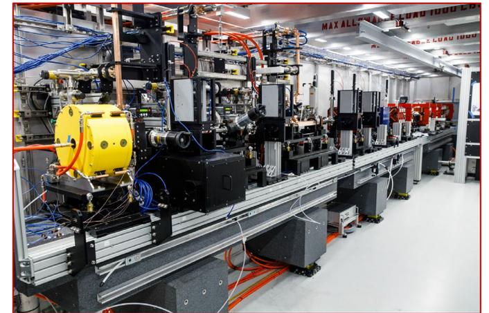
A novel system to generate ultrafast pulses of hard x-rays and coherent soft-x-rays from a compact accelerator design for use in research across biology, physics, materials science, chemistry and other disciplines.
