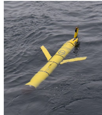
All Global and Coastal Arrays use gliders to collect physical and biogeochemical data to supplement those collected by the stationary moorings. At the Global Arrays, the gliders collect data from the subsurface moorings using acoustic technics and relay the data to shore via satellite. Credit: Sawyer Newman, WHOI.
