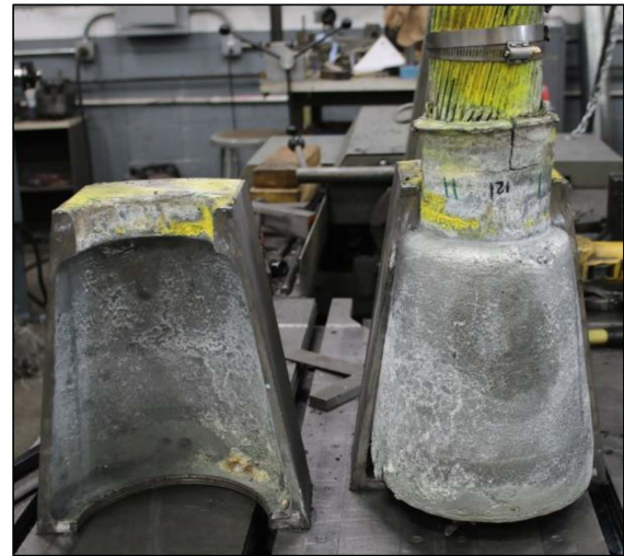
Figure 31: Surface corrosion of B12W_G socket casting (photo: Socotec).
