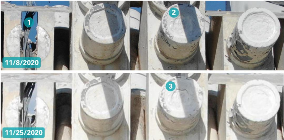
Figure 28: Evidence of socket casting core displacement after second cable failure (photos: NAIC Arecibo Observatory, a facility of the NSF).
