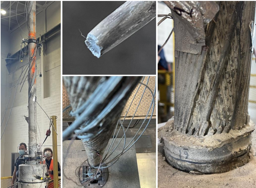
Figure 56: Failed wires in B4S_G socket at end of load test.
