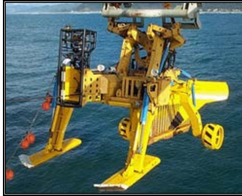
Figure 2-23. Example of a Submarine Cable Plow
