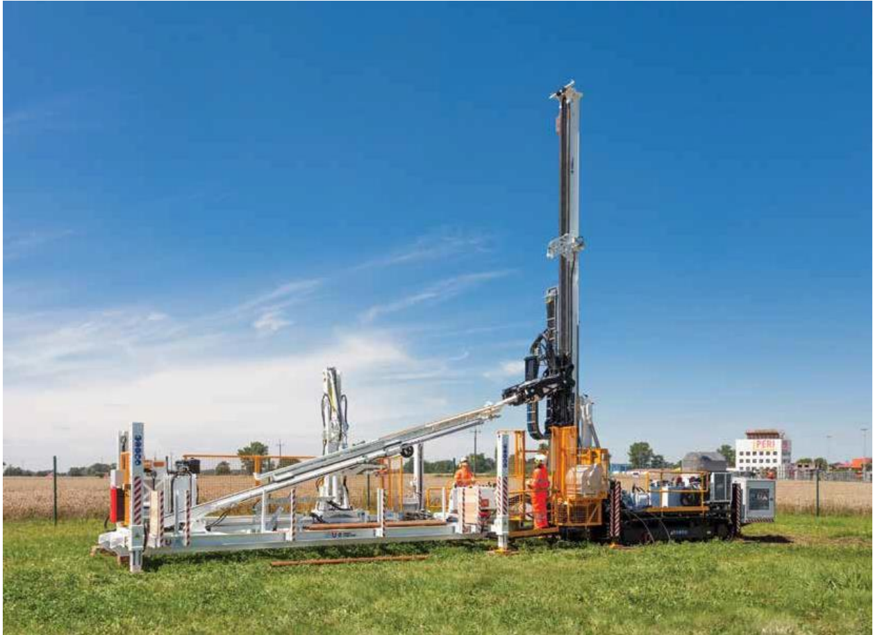
FIGURE A-3. Boart Longyear LF160 Drill Rig, up to 10.6 m high. This land-based mining rig would be temporarily installed on the L/B Robert for the proposed action (Source: Boart Longyear).
