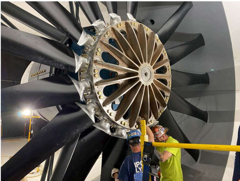
*Figure 2: Aerolab MIT Fan During Assembly*
