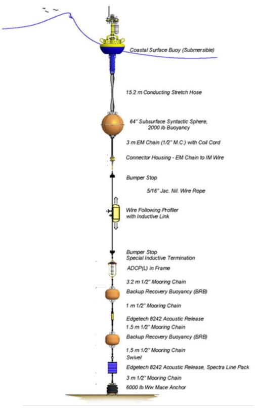
Figure 3. Proposed Coastal Profiler Mooring Design
