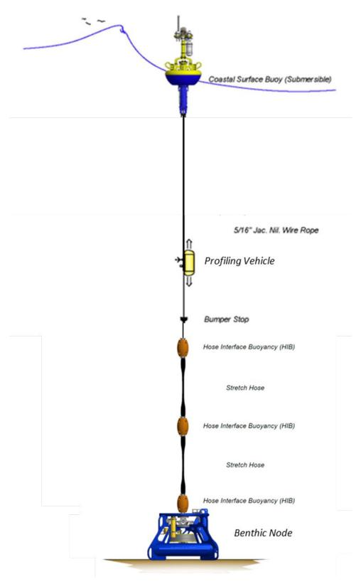
Figure 2. Proposed Shallow Water Mooring Design
