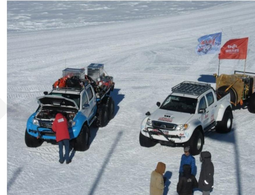
AGILE OVERLAND TRAVERSE. Small overland traverse vehicles have been used in Antarctica in the past and may be a cost and time saving alternative to field flights in crevasse-free areas. Source: NSF, Undated.
