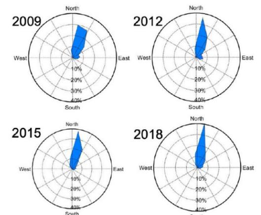
Figure 7.17 South Pole wind roses used for snowdrift modeling.
