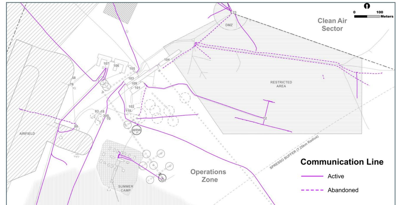
Figure 7.10 Communications Network Core Area
