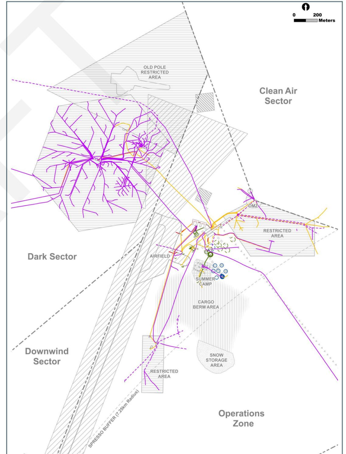
Figure 5.2 APPROXIMATE CABLING MAP. The station area has an overlapping network of cables running under the ice. In this graphic, yellow indicates power lines, blue indicates water lines, green indicates waste piping, purple indicates communications and data cabling. Source, NSF, Undated. Not to scale.
