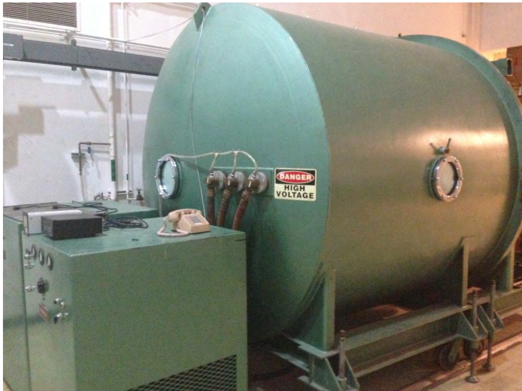
Photo 50: Mirror coating tank inside Dunn Solar Telescope
