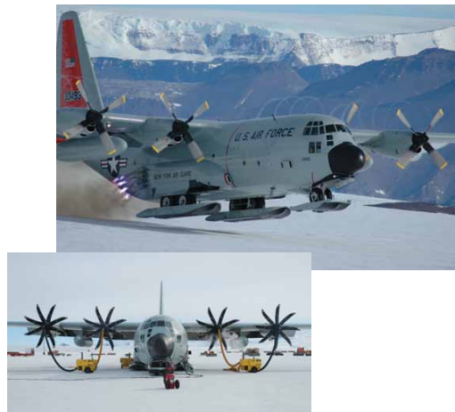
Figure 4.18. (top) A USAP LC-130 aircraft using assisted takeoff. Source: Charles Kaminski. (bottom) An LC-130 with eight-bladed propellers. Source: USAP photo archives.
