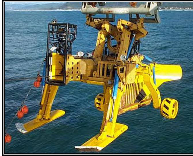
Figure 2-19 Example of a Submarine Cable Plow
