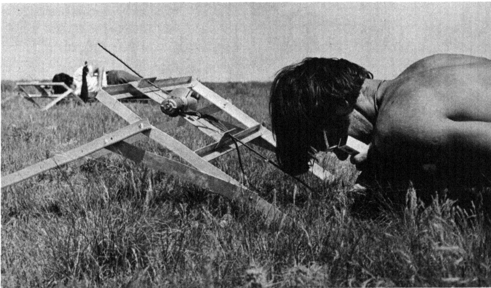
IBP research technician observes motor-driven probe (running diagonally from upper left to lower right), and records all the plants that it touches in its journey to the ground. Resulting data, which reveal utilization of sunlight, are used in computer model of grasslands.
