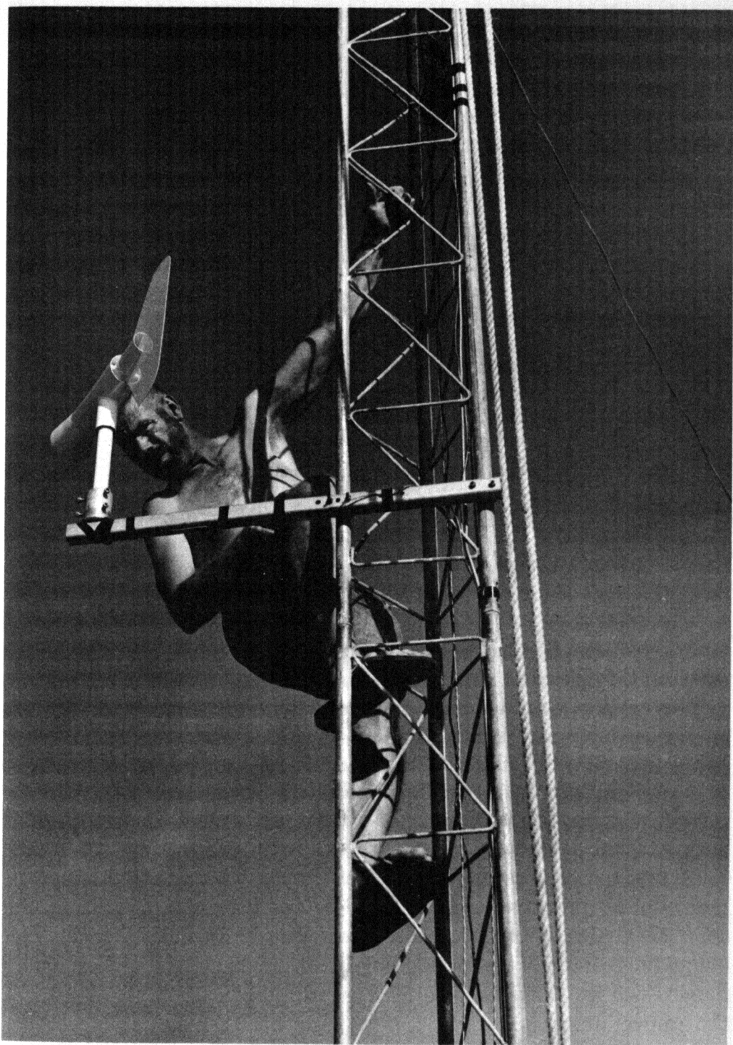
Figure 13.—NCAR technician checks wind speed instrumentation at an observing site on Palmyra atoll during the Line Islands Experiment in the spring of 1967.
