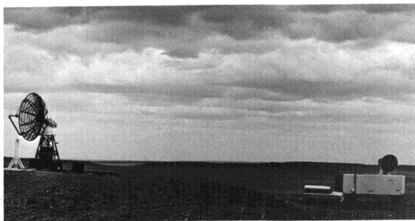
An NCAR radar detects developing hailstorms on the prairies of Pawnee National Grassland, north of Raymer, Colo. (NCAR photo)
