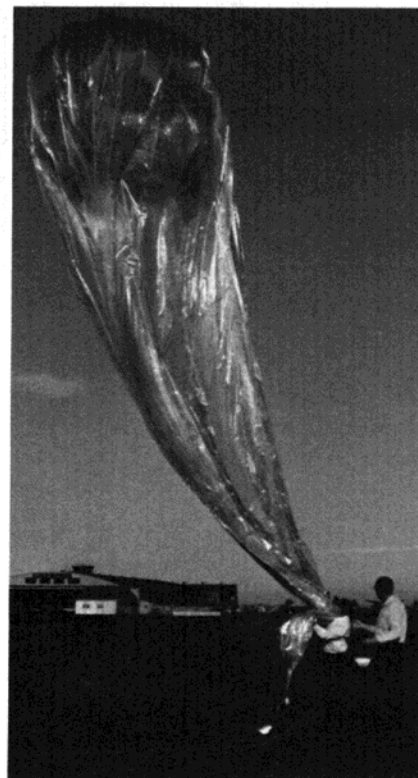
A constant-level GHOST balloon is launched from Christchurch, New Zealand. Balloons such as this, drifting with the wind, will transmit temperature, pressure, and wind data to satellites for relay to ground stations. (NCAR photo)
