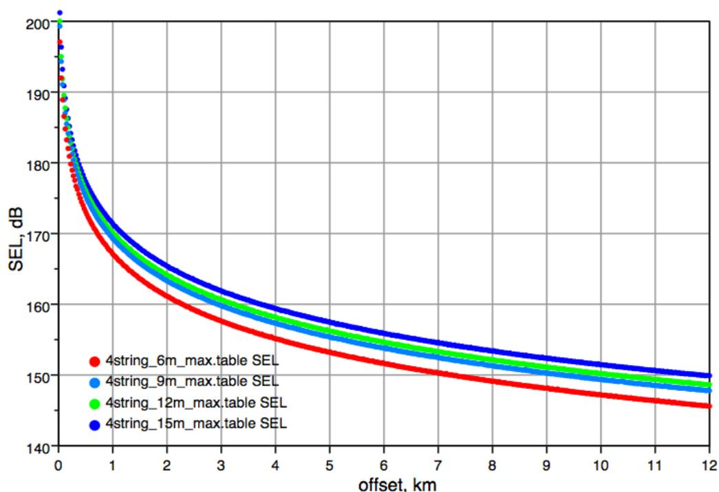
**Figure 6.** Direct-arrival modeling for the *Langseth* maximum 4-string source array as towed at four different depths. Lowest values correspond to the 6-m tow depth used during calibrations. Note that the increase in energy levels is not linear with increases in tow depth.
