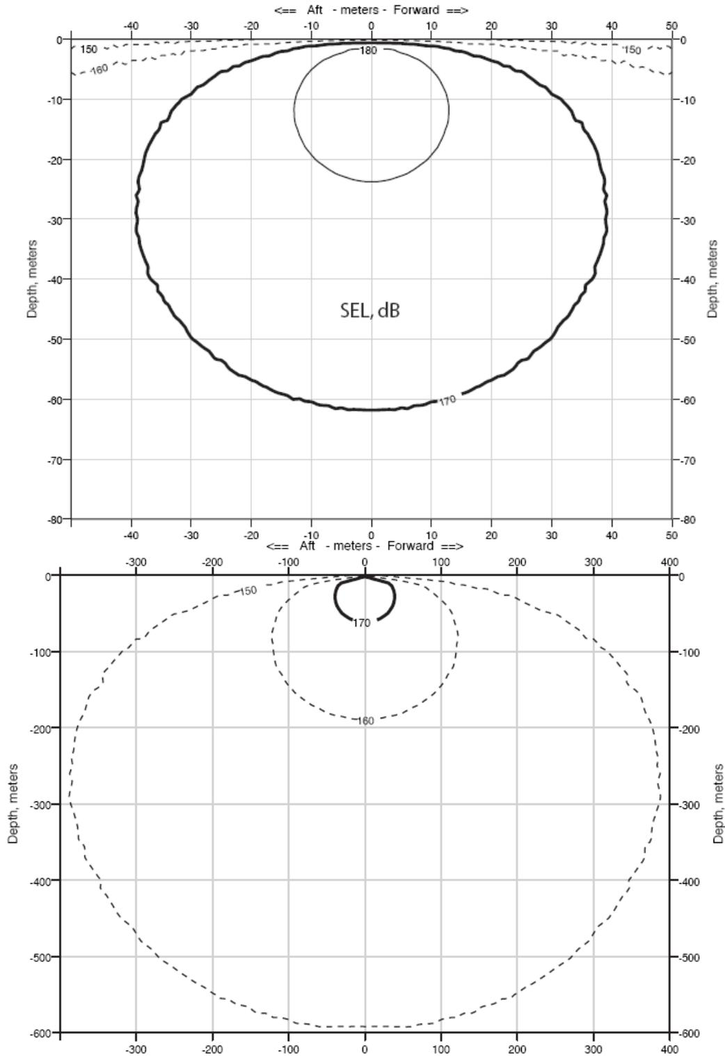
FIGURE 4. Modeled received sound levels (SELs) in deep water from a single 40-in<sup>3</sup> airgun, which is planned for use as a mitigation airgun during the surveys in the northeastern Pacific Ocean, 11 June–23 July 2012. Received rms levels (SPLs) are expected to be ~10 dB higher.
