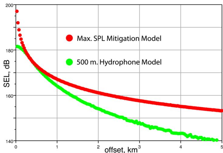
**Figure 2.** The modeled sound exposure levels along the “hydrophone depth” and “maximum SPL” lines drawn in Figure 1. The lower, green line should be compared to the calibration results, while the upper red line has been used to establish mitigation radii.
