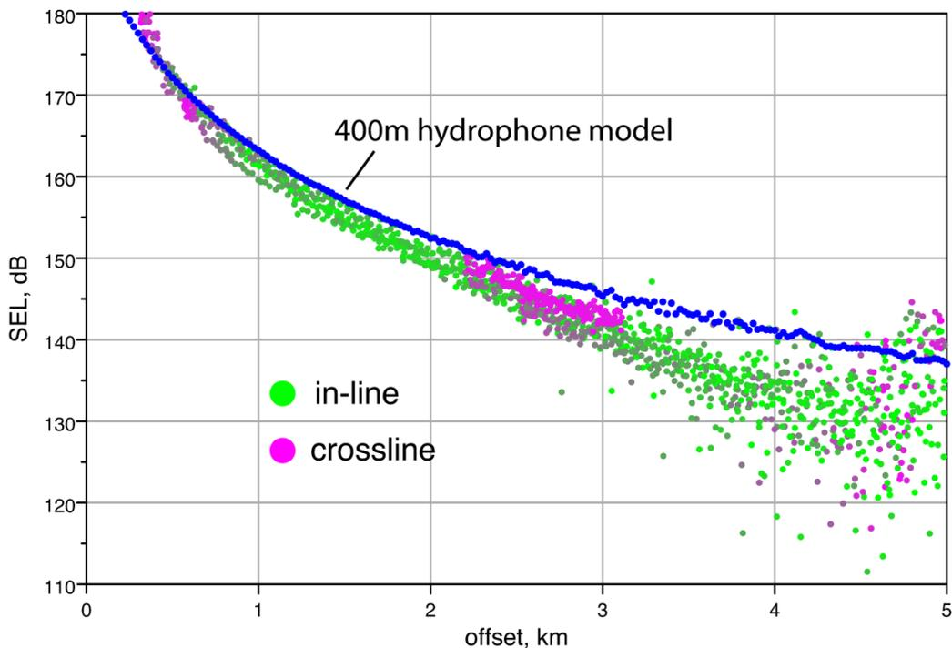
**Figure 4.** Energy flux density (SEL) values for direct arrivals at the slope site. In-line and cross-line aspects are color-coded. The 4-string model with 6-m tow depth and receiver depth of 400 m is shown for comparison. The model is only exceeded by the data at small offsets, and at large offsets where the direct arrival windowing started to fail.
