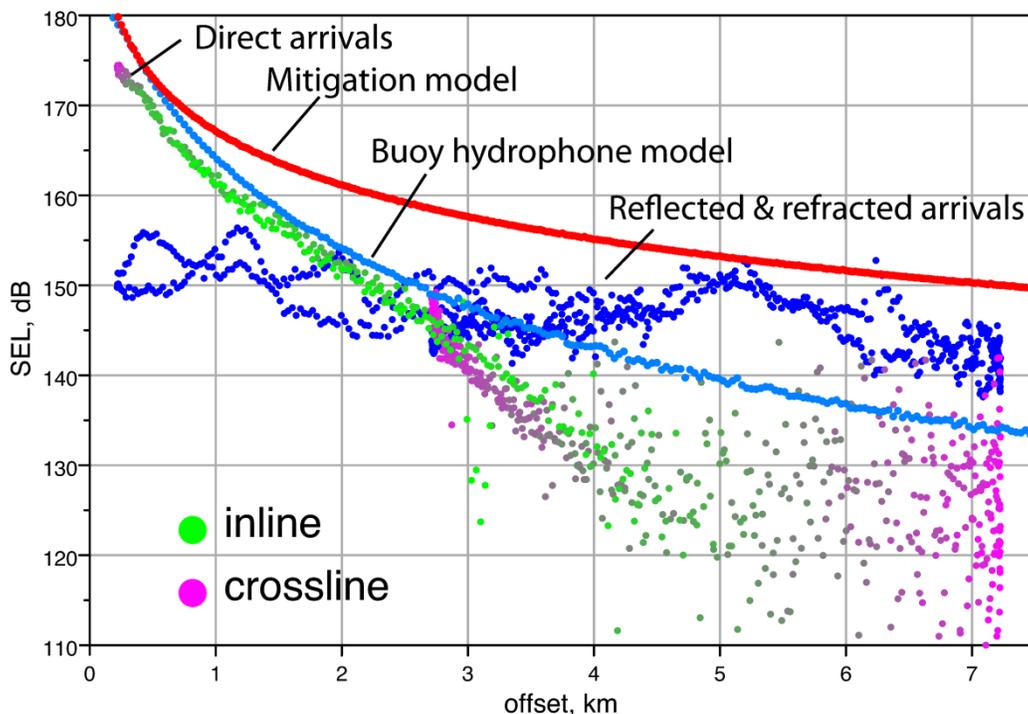
**Figure 3.** Energy flux levels for direct and reflected/refracted arrivals from the 4-string array at the deep calibration site. The maximum SPL, or “Mitigation” and “Buoy hydrophone” models do not include bottom interactions. The Buoy hydrophone model matches the observed direct arrival data very well, although it consistently over predicts amplitudes by a few dB.
