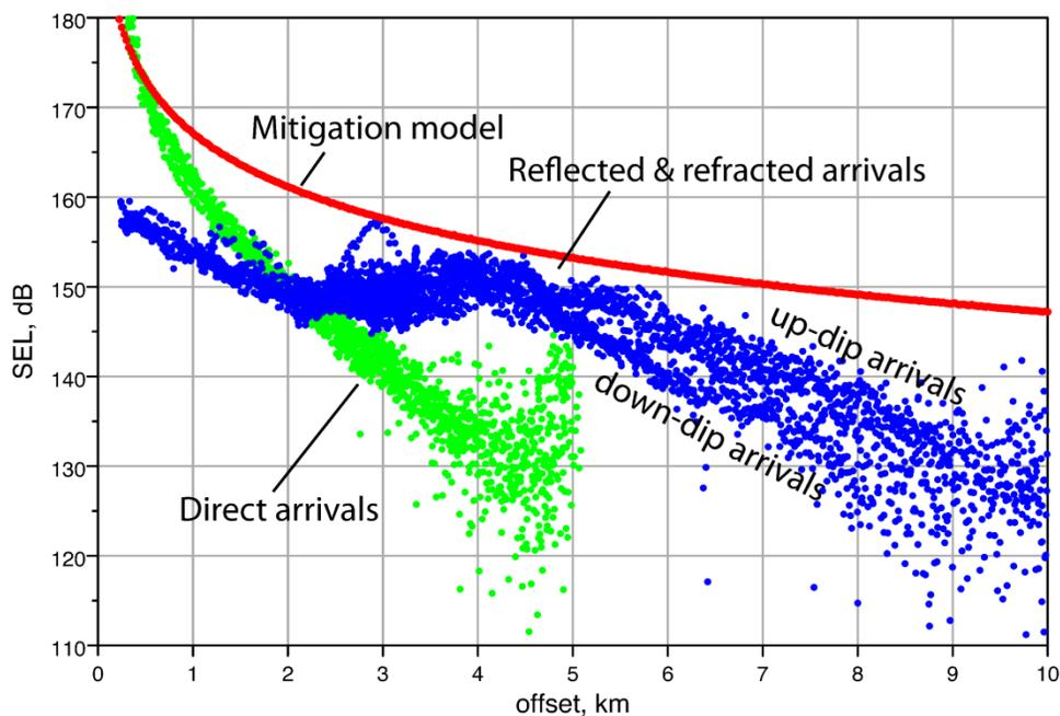
**Figure 5.** As in Figure 3, measured levels for seafloor reflected and sub-seafloor refracted arrivals are superimposed on the direct arrival values. Because the water is shallower at this site, the critical distance is 4 km, rather than the 5 km observed at the deep site. All observed levels (except at very near offsets) fall below the mitigation model predictions.
