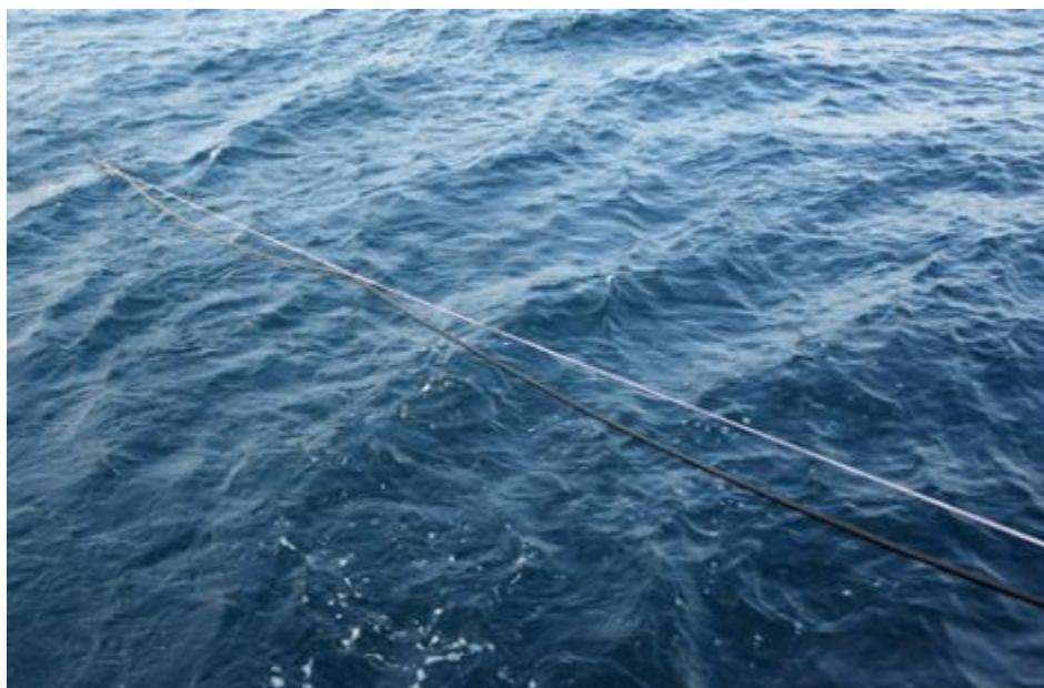
Figure 2. Hydrophone deployment method using a taut line to absorb the tension of a weighted depressor affixed to the hydrophone cable to give it sufficient towing depth to drop below the gun umbilicals and streamer lead-ins.
