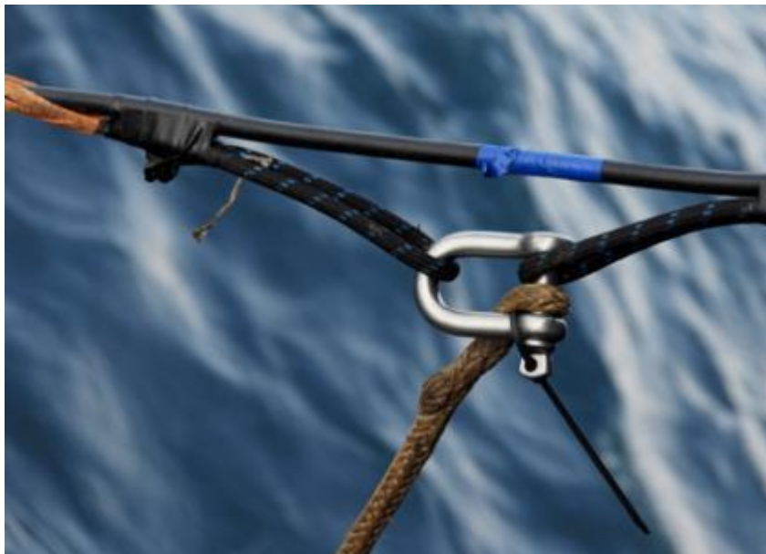
Figure 31. Two chinese fingers on the hydrophone cable 20m ahead of the first hydrophones. Shackle and line attach to the depressor weight
