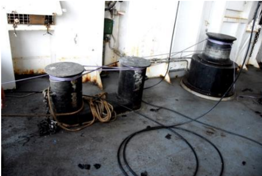
Figure 32. Depressor tow line deployed from capstan alongside PAM hydrophone cable which is deployed from the deckhead winch
