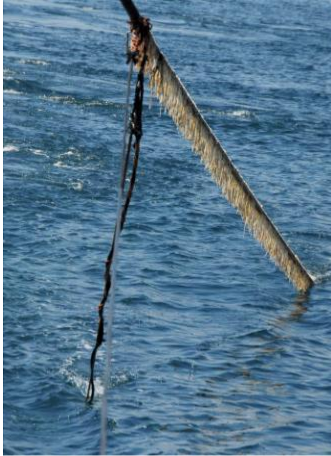
Figure 33. Hydrophone cable and depressor tow line wrapped around inner port side lead-in on 2 May.
