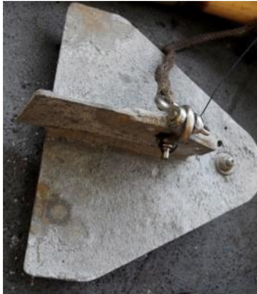
Figure 28. Depressor weight towed from a line and attached to the hydrophone cable to achieve sufficient towing depth to get below the gun umbilicals and streamer lead-ins
