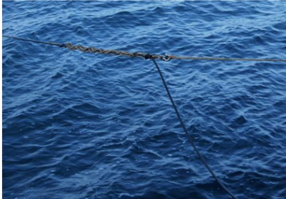
Figure 30. New PAM cable deployment set-up used after 2 May where depressor and it's tow line are eliminated. Cable is deployed by itself off PAM winch with diverter rope from port side barovane platform attached by chinese finger to pull the cable off to the port side
