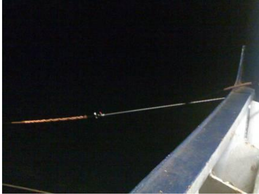
Figure 4. Hydrophone cable secured by a yale grip to the port sponson
