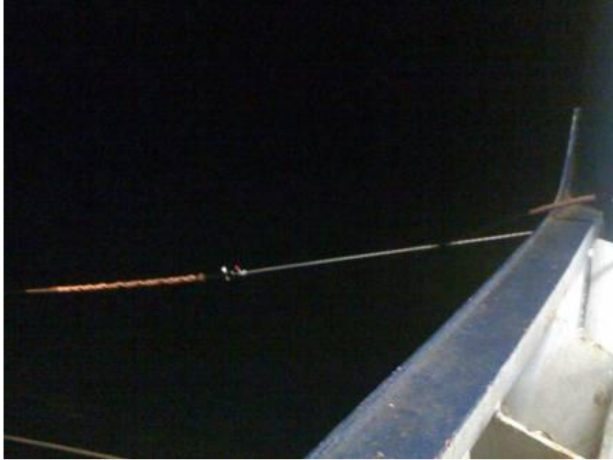
Figure D.17: Hydrophone cable secured by a yale grip to the port sponson.
